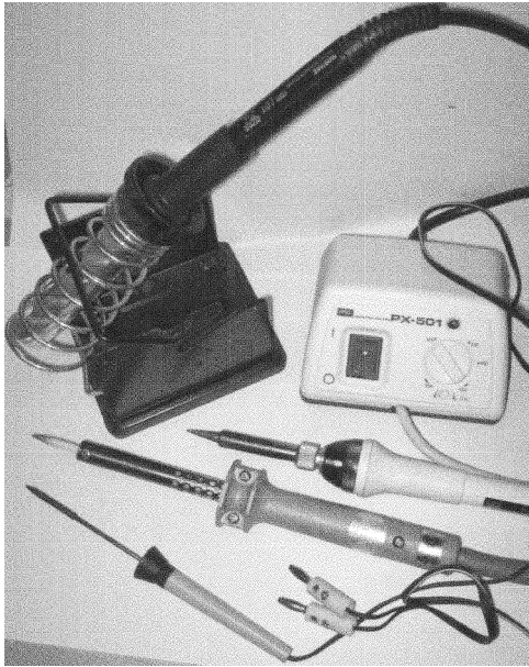
Figure 9.2: Soldering irons, from back to front: professional soldering iron with soldering stand, low-cost soldering station, basic iron, and 12 V iron.
