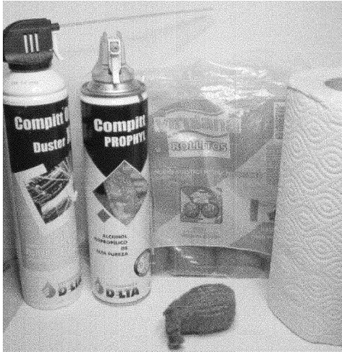
Figure 3.7: Cleaning tools from left to right: “compressed air”, isopropanol, steel wool, and paper towel.
