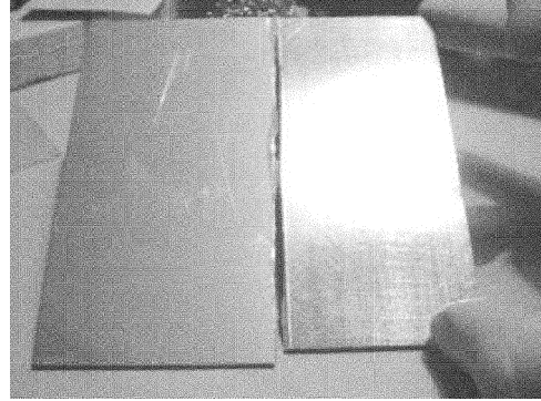
Figure 3.8: Before cleaning (left), oxidation makes the copper look dull. After cleaning (right), the copper is shiny.
