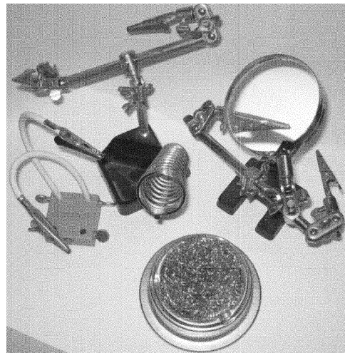
Figure 15.1: Helping hands, from left to right: flexible arms, regular model with solder iron stand and a sponge receptacle, and a regular model with a magnifying glass. Below, there is a tip cleaner with bronze wool.
