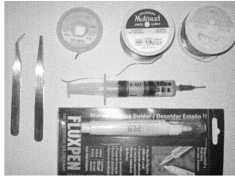
Figure 9.3: Soldering tools. Top row, from left to right: desoldering braid, regular solder, and “eutectic” solder. Bottom row: angled and flat tweezers, flux syringe and pen.
