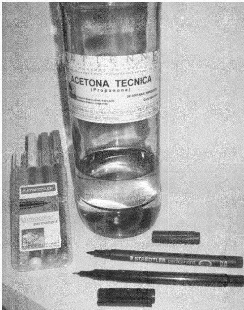
Figure 5.7: Toner touch-up and removal: bottle of acetone, permanent marker, and an etch-resist pen.
