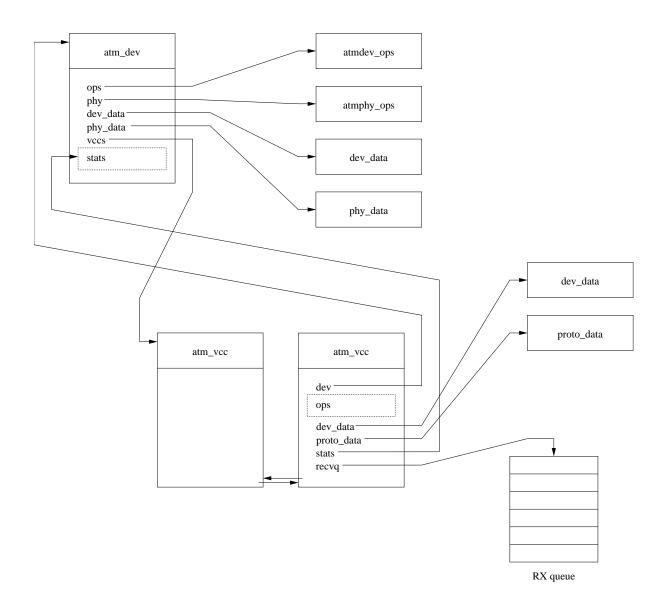
Figure 2: Device and VC data structures.
